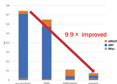
GPU (OpenACC or CUDA) vs CHARM (CUDA+OpenCL or MHOAT) ⇒ MHOAT is the best with 10 \times speed of OpenACC GPU
