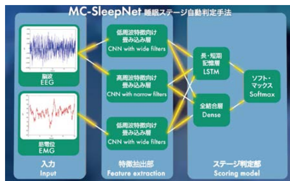
Scheme for an automatic sleep stage determination method using deep learning
