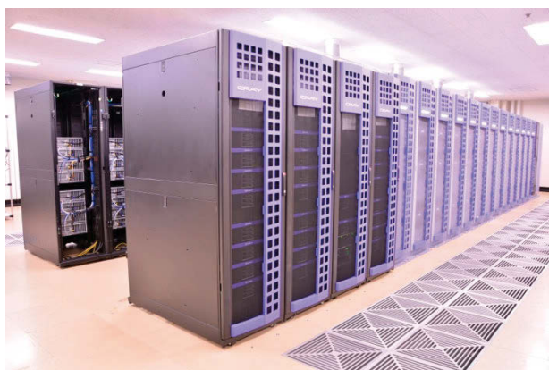
Fig. 2 Overview of HA-PACS Base Cluster and TCA part (five racks of front side are for TCA part and others are for Base Cluster)
