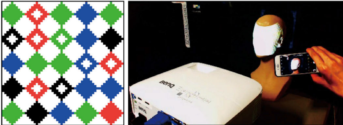
Figure 12. The structured light pattern used for calibration (left) and the experiment setup (right)
