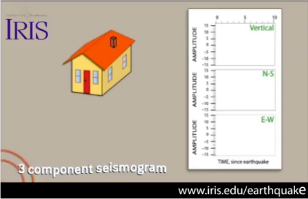
3-Component Seismogram Records Seismic-wave Motion
