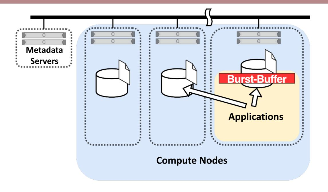
Node-local burst buffer is expected to be a promising caching layer for a distributed file system. To design a node-local burst buffer, we evaluate current solutions including Gfarm/BB, BeeOND, and Octopus using NVMe SSD and NVRAM.
