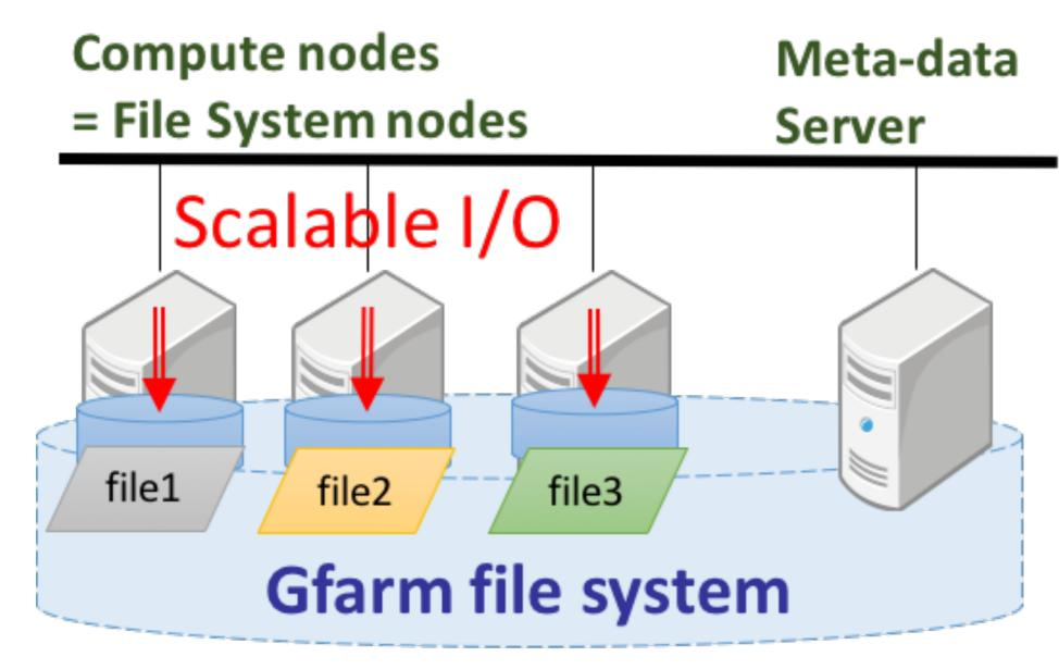
It is a Node-local burst buffer and a Grid file system. Features include
