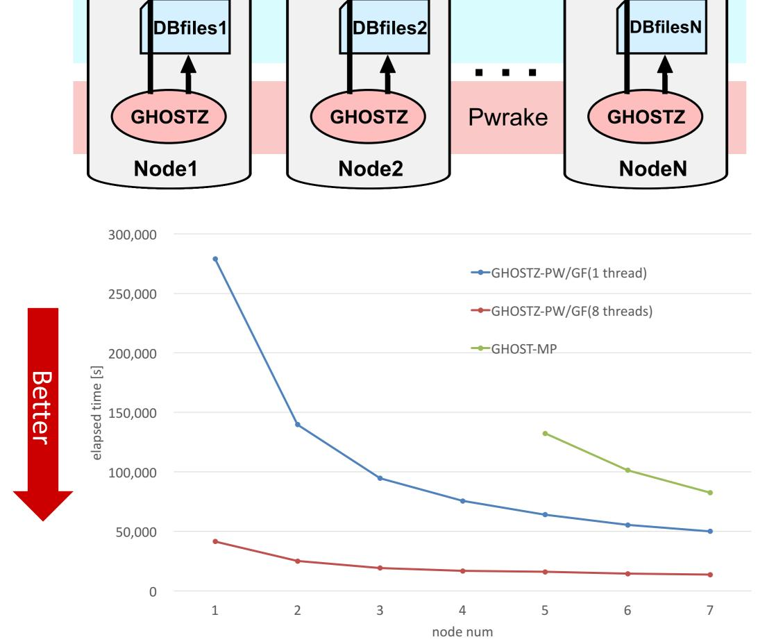
In recent years, acquired genomic data size is rapidly increasing, which results in memory shortage in a cluster node and long execution time. GHOSTZ with Pwrake/Gfarm solves these issues using node-local storage and locality aware workflow execution. It outperforms GHOST-MP 6x times in an alignment step when using 7 nodes.
