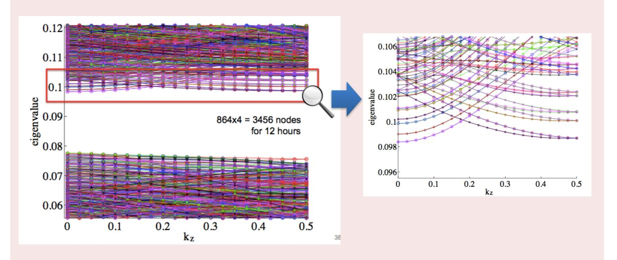
Band structure of silicon nanowire of 9,924 atoms. (matrix size = 8,719,488, Number of cores = 6,144)
