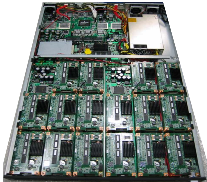
Cluster Unit of MegaProto/E with 16 CPUs
