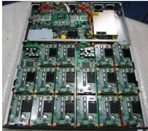
Low-Power and High-Performance Cluster Unit “MegaProto”
