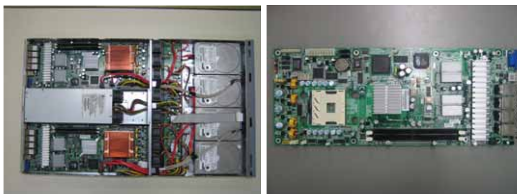
Figure 5.2: PACS-CS motherboard (left) and mount on 1U chassis unit (right)
