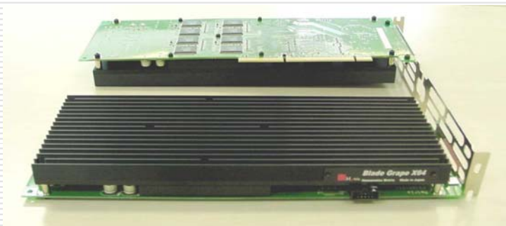
Blade-GRAPE board (136.8GFLOPS)
