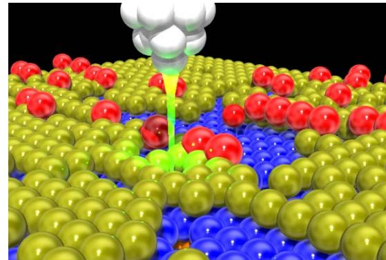
Tunneling current flowing between STM tip and sample surface
