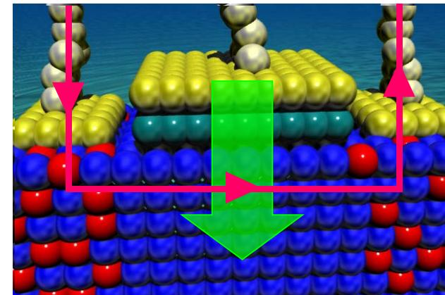
Electron transport between source and drain of semiconductor device
