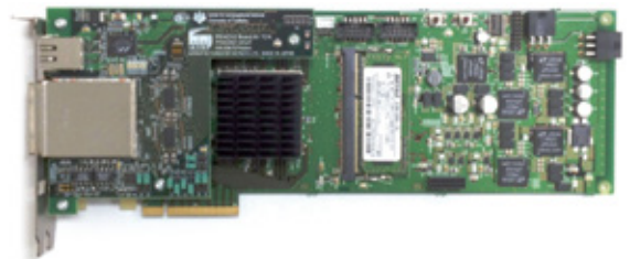
Fig.1 Prototype PEACH2 chip test board for TCA environment use
